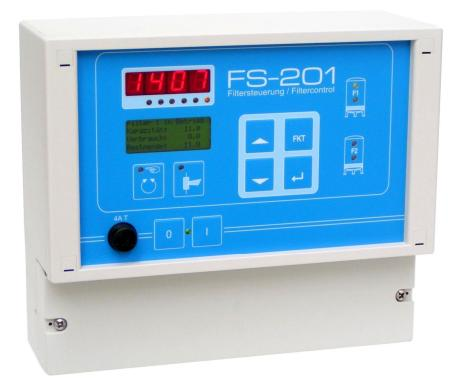
The FS-201 filter control unit serves to control a one- or two-filter system equipped with pilot distributors or central control valves. The valve types are selected by means of the parameter settings and the FS-201 automatically adapts to the filters selected as the function progresses. Both decarbonisation filters as well as gravel filters can be controlled.
