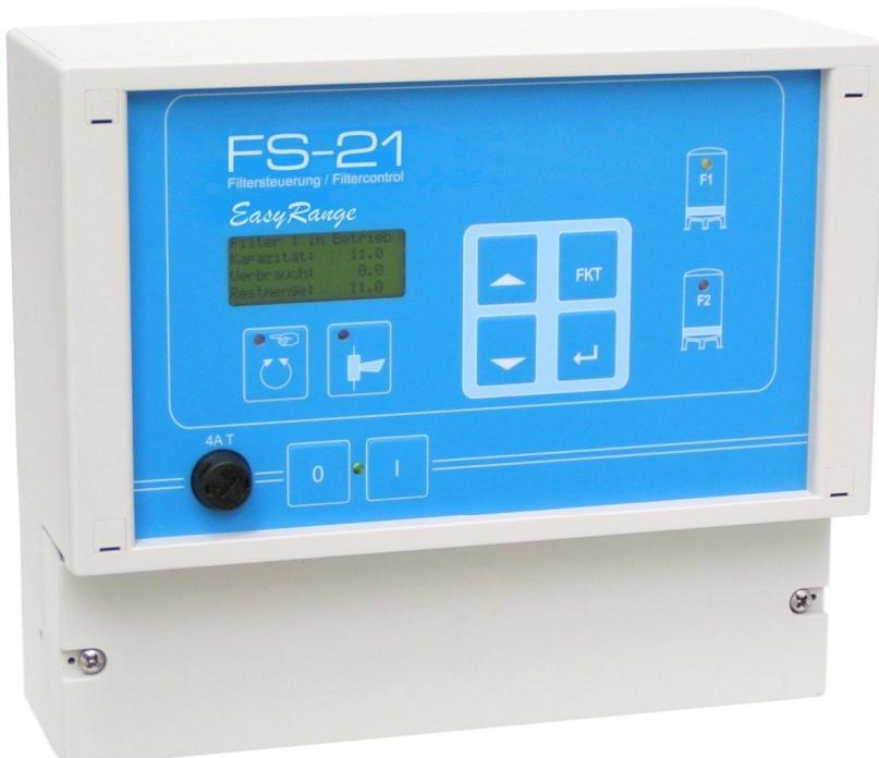
The FS-21 Filter Controller performs the basic tasks for controlling a single or double filter unit with pilot distributors or central control valves. The valve types are selected via configuration and the FS-21 adapts automatically to the selected valve type during the course of operation. Both decarbonisation filters and gravel-packed filters can be regulated. For more complex applications and an expanded range of functions, we recommend the use of our FS-201 filter control.
