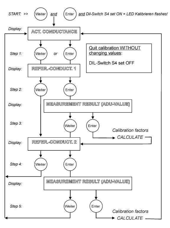
Taking over of calibration values (at any time) by simultaneously actuating of both keys while DIL - Switch S4 is set ON! Thereafter switch S4 to OFF!
