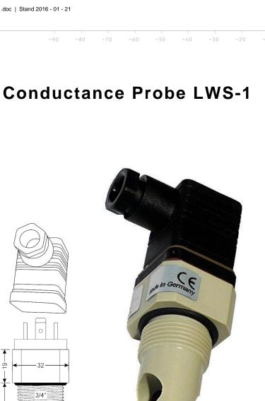
The LWS-1 Conductance Probe is a 2-electrodes conductivity measuring cell. It is available in three variants: without - and with temperature compensation by means of Pt100 temperature measurement, as well as for an extended temperature range up to 120 °C (see Technical Data / Ordering Information ).
